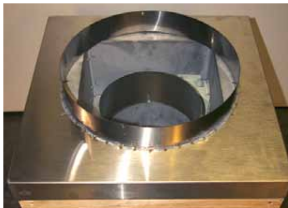
Figure 4d. (Installed Stainless steel cover)
